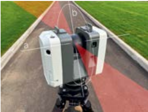
Fixed-position laser scanner rotation during a survey (Adobe stock)
