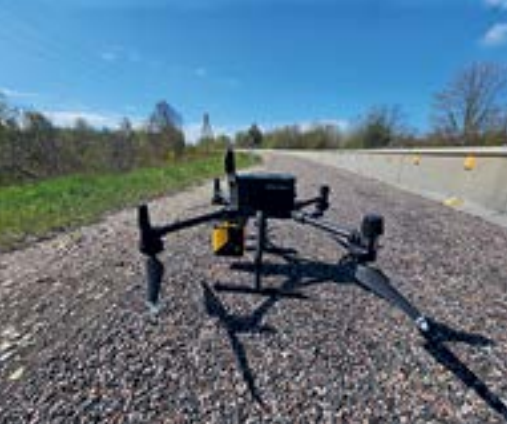
Unmanned aerial vehicle equipped with a LiDAR sensor (author: M. Rutkovskis)
