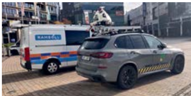
MLS device equipment on a road vehicle (author: M. Kakko)
