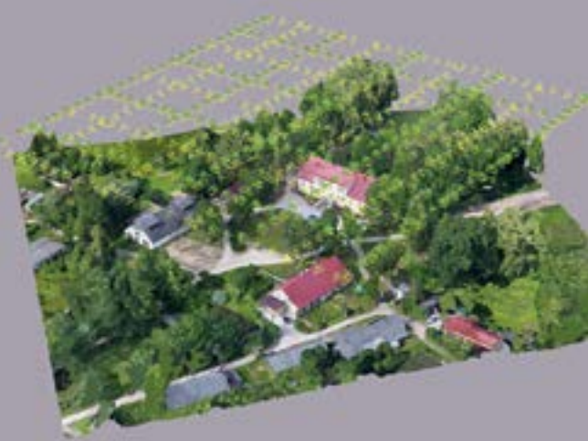
Arrangement of photographs above an object for producing an area model (author: M. Kaļinka)
