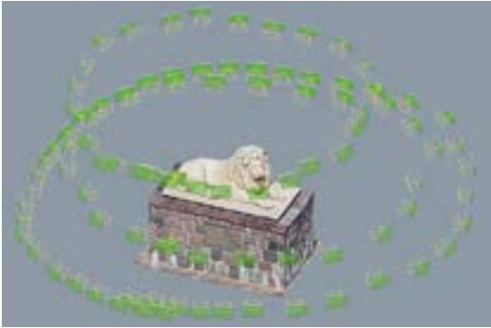
Layout of photographs around an object for a 3D survey (author: M. Kařinka)
