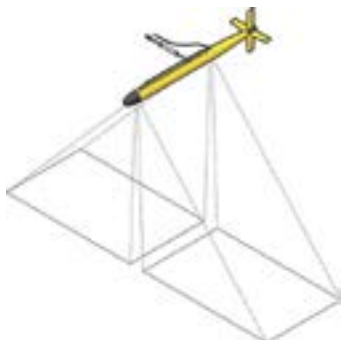
Side-scan sonar surveying principle (Adobe stock)
