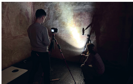
Photographing a mural using the RTI method. Photo: Gunnar Almevik
