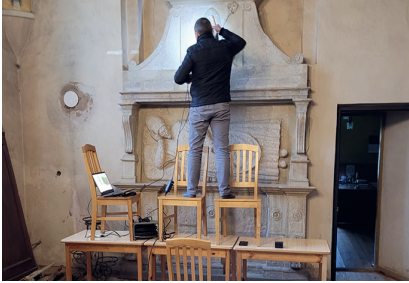
Surveying process using a 3D handheld scanner (author: A. Åbele)
