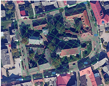
Flight plan diagram for photographing a city block with a UAV (author: J. Heinsbergs)
