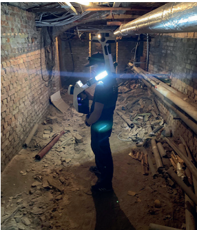
Working with portable laser scanning equipment in darker spaces (author: J. Heinsbergs)
