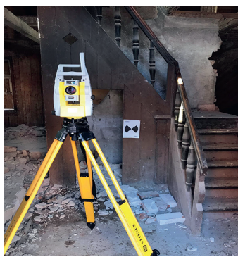
Placement of laser scanning markers on an object (author: J. Heinsbergs)
