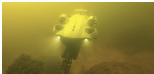
Surveying and photographic recording of a shipwreck using an underwater drone (author: K. M. Molls)
